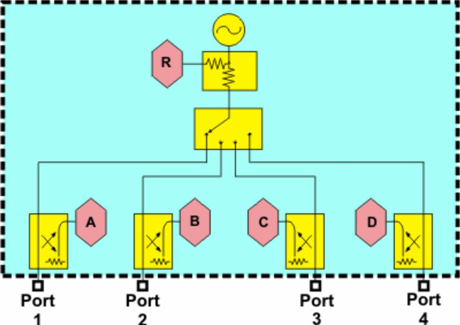
**N5230A Option 145 or 245 Configurable Test Set and Extended Power Range**
